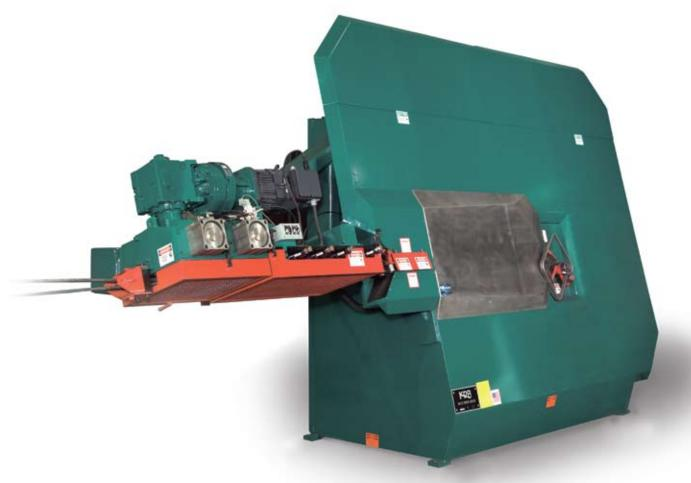
The Coil Form 1020 C processes dual strand #3 (10mm) through #5 (16mm) straight or coiled stock and single strand #6 (20mm) from straight stock. This Automatic Stirrup Bender has been designed for maximum flexibility with a straightening system that can be removed to allow straight bars to be processed when the application calls for this. Epoxy coated rebar can be processed with
