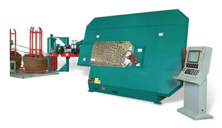
The Multi Form 1020 M ES automatically bends and shears deformed reinforcing steel dual strand #3 (10mm) through dual strand #5 (16mm) from coiled stock. The straightening system is controlled from the operator's station without the use of tools. The straightening rolls can be preset, recalled and changed with the push of a button, for all bar sizesvia Servo Driven Linear Actuators.
