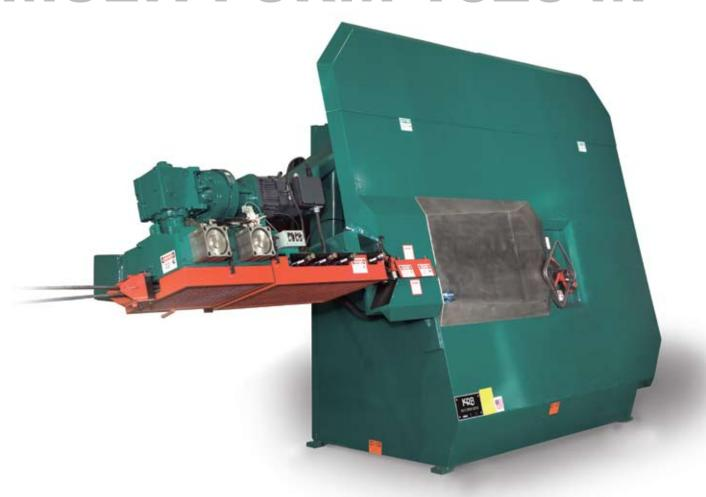
The Multi Form 1020 M processes dual strand #3 (10mm) through #5 (16mm) straight or coiled stock and single strand #6 (20mm) from straight stock. This Automatic Stirrup Bender has been designed for maximum flexibility with a straightening system that can be removed to allow straight bars to be processed when the application calls for this. Epoxy coated rebar can be pro-
