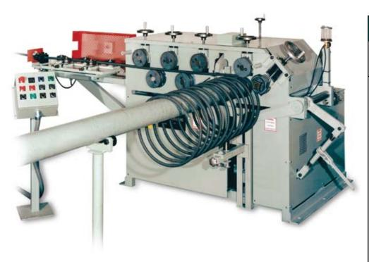
KRB SpiralMatic 722HD spiral machine complete with heavy duty coil cradle will spiral rebar up to #7 (22mm) bar; grade 60 or 65kg/mm2. Special features of 722HD not found on all spiral machines include:
