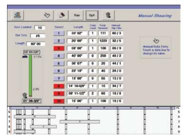
Manual multi-cut allows you to enter up to 10 lines & optimize; graph at bottom of screen shows visual binning of bar in pocket locations.
