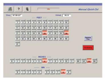
Manual quick cut is a single cut & unload stop entry for manual cutting similar to traditional toggle switch control consoles. This feature is perfect for "tags only" cutting. With minimal key strokes, the operator errors can be eliminated, compared to other shearline controllers.
