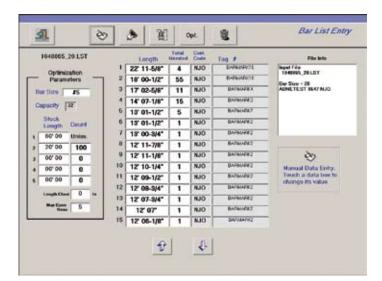
The operator can scan, manually input or download a cut list and optimize before cutting. Allows for 100 lines of entry. Will optimize up to 5 different stock lengths. Direct downloading of an optimized list.
