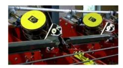
The Arm-Tec SpinMaster is a one-man operated machine for high capacity production of rollmats in a non-welding process, which will make it possible to handle any type of reinforcing steel, even galvanized, stainless or epoxy coated rebar.
