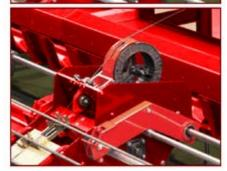
The Arm-Tec SpinMaster BF fabricates non-welded rollmats which expedite placing and tying in horizontal reinforcing applications. Because there is no welding, epoxy-coated, stainless and galvanized rebar, as well as black rebar, can be spaced and prewired to the customer's exact specifications. Simply roll them out and pour your slab!
