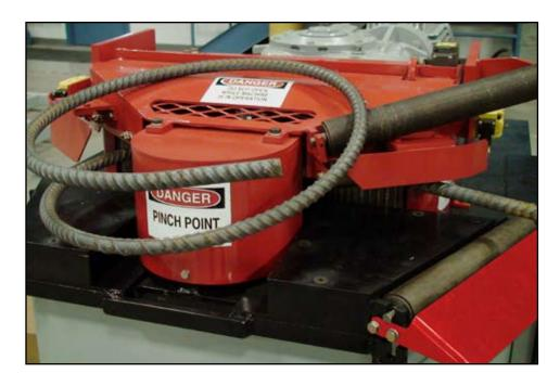
The KRB 11M Radius Bender is designed to radius most rebar without the need to pre-bend the end of the bar. Keeping the operator's hands away from the forming rolls allows safe operation.
