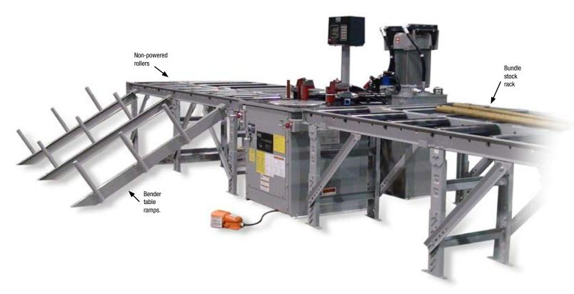
Along with our quality table benders, KRB offers a robust and flexible line of bender tables. Available in 3m sections and in two different styles, powered and economy, we can customize the right solution for you. Our economy tables (pictured above) ease operator fatigue and repetive motion injures. Our economy tables offer a solid, cost effective option.
