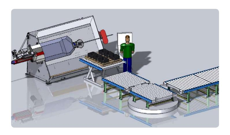
The KRB Stirrup Conveyor allows stirrups to moved away from the bending area and staged to awaiting trucks for loading.
